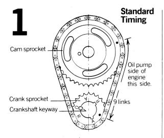
Rotate engine until No. 1 piston is Top Dead Centre (T.D.C.) compression stroke. No. 1 piston is located at front of engine on drivers side. Assemble crankshaft sprocket, camshaft sprocket and chain so that zero timing dots are positioned as shown above. (9 links between dots).
