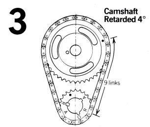
Same as for instruction No. 1, but fit crankshaft sprocket keyway marked 'R' to crankshaft and align Tooth marked 'R' on crankshaft sprocket and timing dot on camshaft, so there are 9 links between them.
