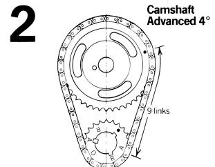
Same as for instruction No. 1, but fit crankshaft sprocket keyway marked 'A' to crankshaft and align Tooth marked 'A' on crankshaft sprocket and timing dot on camshaft, so there are 9 links between them.
