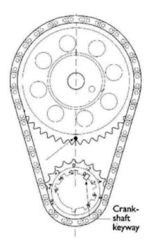
**Warning:** Do not use the keyway marks to time engine. Always align the crank gear tooth timing marks to cam gear timing mark.
